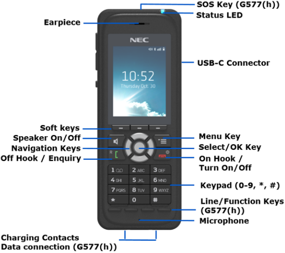
Figure 4: Elements of the G277/577 (Front View)
